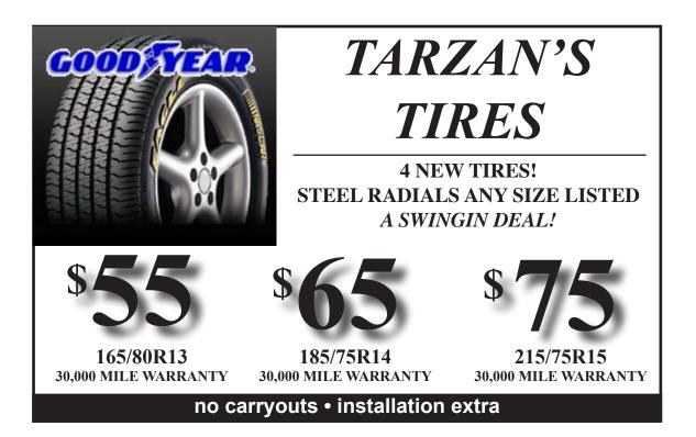
Tires are sold according to the diameter of the wheel or rim. (The last 2 numbers are the diameter.) When these tires are added to the wheels, the total diameters become about 23", 25", and 27" respectively
